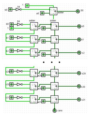
We then simplified the circuit by removing the adder for 1 and instead simply flipped the signals from b and added 1 to the adder that takes the input for a0, thus resulting in the following simplified circuit:
