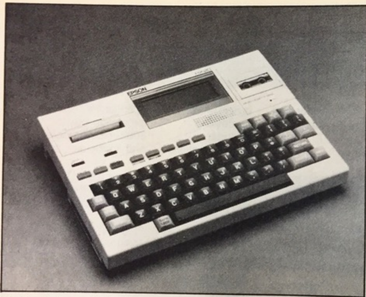
Photo 3: Space limitations on the front panel forced the designers of the Epson HX-20 to use a 20-character by 4-line display.
