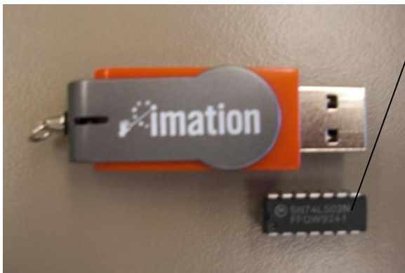
Figure 7. Quad 2-Input NOR Gate 74LS02 Compared to a USB Flash Drive.
