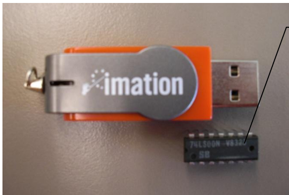
Figure 8. Quad 2-Input NAND Gate 74LS00 Compared to a USB Flash Drive.
