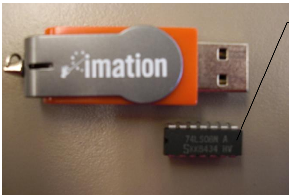
Figure 3. Quad 2-Input AND Gate 74LS08 Compared to a USB Flash Drive.
