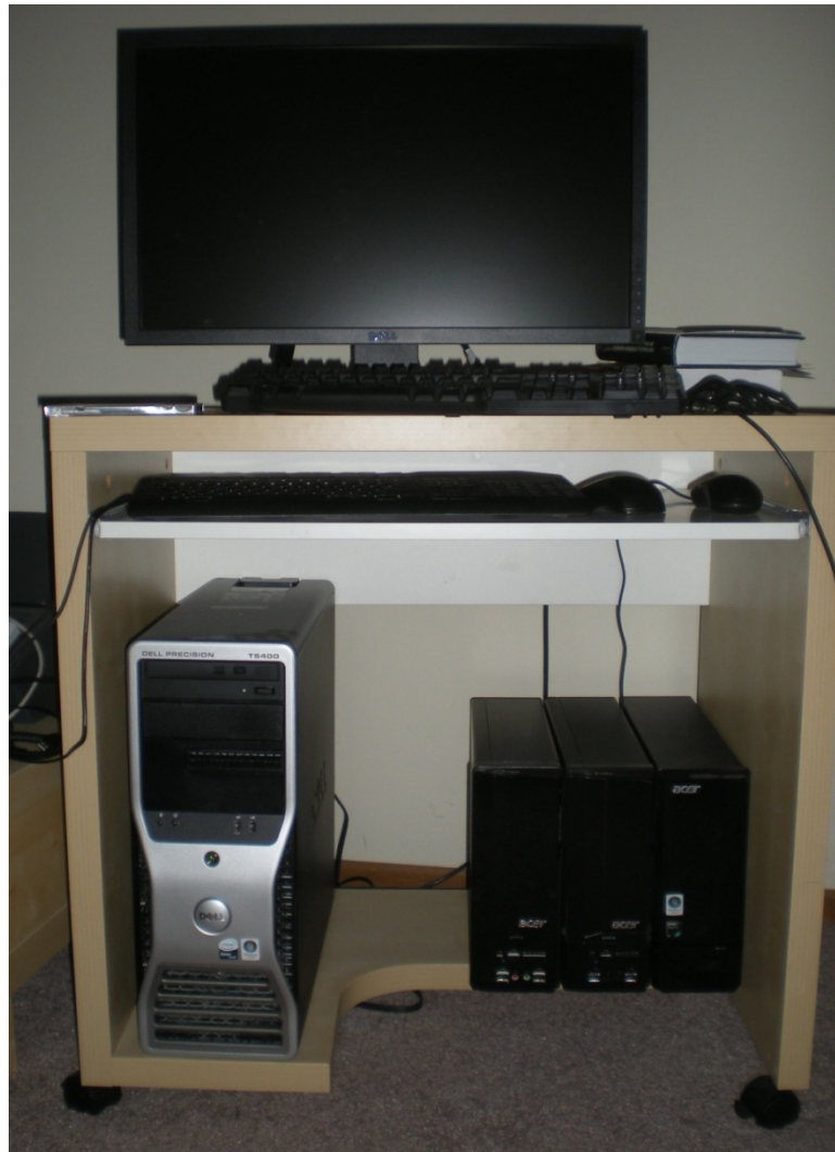
Figure 1. Hydra, a miniature cluster with one master PC and three nodes.
