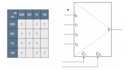
My work for part one of problem 1 is shown below. For each CD row I connected the C & D binary value to its matching f (i.e. 11 maps to  $f_3$ ), and set the input to be the defining feature of that row of the Kernaugh map.
