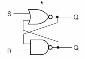
To solve this problem, I first tested if the circuit above was a latch. I did this test by using a state table to test if changes in S and R caused  $Q_i$  and  $Q_j$  to change in a predictable way. If they changed in a predictable way, (i.e. whenever S and R switched values,  $Q_i$  and  $Q_j$  switched values as well), this would indicate that the values of S and R were being stored and remembered. My state table is found below.
