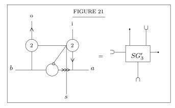
When SG' is on, a stimulus needs one period  $\tau$  to get from b to o, i.e. to  $L_o$  (cf. 13.3 and the end of this Section 13.4), and one to get from  $L_i$ , i.e. from i (cf. Figure 20) to a—that is, it takes  $3\tau$  from b to a. It is desirable that the timing should be the same when SG' is off, i.e. when the stimulus goes via  $\bigcirc$  from b to a—hence a triple delay is needed on  $\bigcirc$ .
