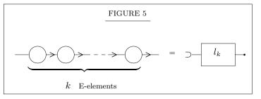
and provide it with such terminal equipment (at both ends, possibly connecting them) as may be required in each particular case. This simple line is shown again in Figure 5. Terminal equipment, which will normally cycle the output os at  $l_k$  's right end back into the input at its left end, but upon stimulation at s suppress (clear) this returning of the output os and connect instead the input with the line rs, is shown in Figure 6.
