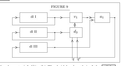
clearly have to contain dl like elements (cf. {}). (b) The k (delay lengths) of the dl I dl III. These too have certain functions of synchronization: Each time when the adder functions (that is in each interval it-ft) the multiplicand and the partial product sum (that is the outputs of dl I and of dl III) must be brought together in such a manner that the former is advanced by t (moved by one position to the right) relatively to the latter, in comparison with their preceding encounter.
