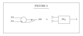
It should be noted that this ml corresponds to the actual vacuum tube trigger circuits mentioned at the beginning of 5.1. It is worth mentioning that ml contains one E-element, while the simplest trigger circuits contain one or two vacuum tubes (cf. loc. cit.), in agreement with the estimates of 6.5.
